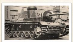
The Soviet SU-76i self-propelled gun was based on captured German Panzer III and StuG III chassis, armed with a ZiS-5 76.2mm gun.
